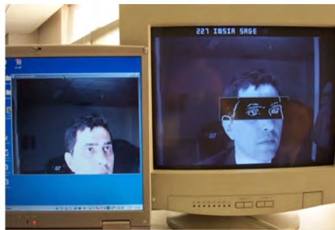
Figure 12.4: Region of Analysis in the DAM System. The image is shown by reading intermediate signals directly from the board on a laboratory, as they are not accessible in the real, in-vehicle configuration.
