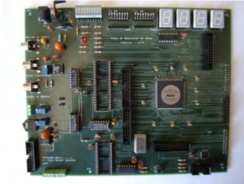
Figure 12.1: Prototype board for the DAM.
