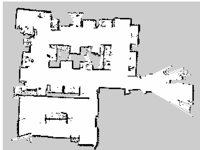
Figure 8.3: Map of Sala de Calculo generated by the Higgs's SLAM system
