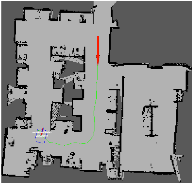
Figure 2.13: A motion path generated for a mobile robot. The goal position and orientation is represented by the red arrow
