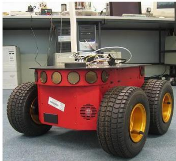
Figure 4.2: The Pioneer 2-AT8 platform used to implement the RCT Higgs Robot
