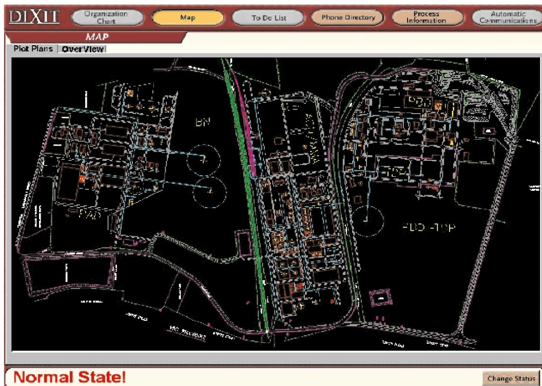
Figure 45: RiskMan Emergency manager user interface. The figure shows the navigation map used to focus on specific areas of the chemical complex.
